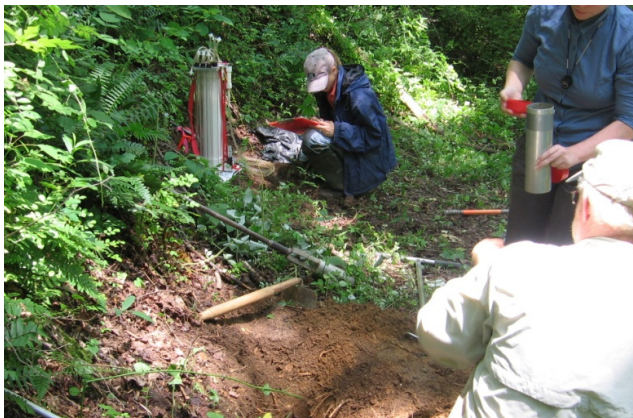
Youth Advocacy Intern, Tiffany Liner (holding canister), assists N.C. Geological Survey Landslide Team members Rick Wooten and Jennifer Bauer, measuring shear strength of soil in a landslide investigation.
